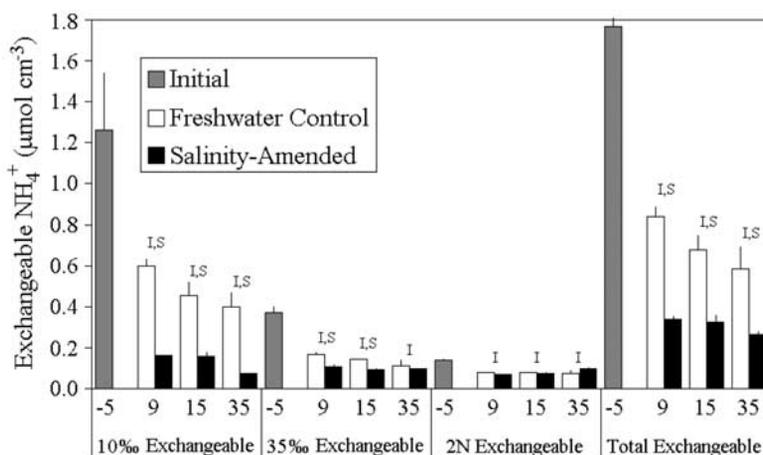
**Figure 5.** The 10‰, 35‰, 2N, and total exchangeable  $\text{NH}_4^+$  from initial sediment cores (3- to 5-cm depth) and control and salinity-amended flow through reactors sampled on days 9, 15, and 35 (mean  $\pm$  standard deviation,  $n = 2$ ). Statistical differences ( $p < 0.05$ , pair wise) between reactors and initial sediment (I) and between control and salinity-amended reactors (S) are noted.
