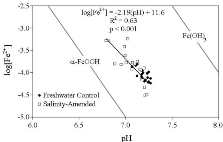
**Figure 4.** Diagram of pH and  $\log[\text{Fe}^{2+}]$  concentrations of water exiting control and salinity-amended flow-through reactors. The stability isopleths for goethite ( $\text{FeOOH}$ ) and amorphous iron oxides [ $\text{Fe}(\text{OH})_3$ ] are indicated.
