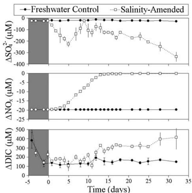
**Figure 3.** Net change in concentrations ( $\pm$  standard deviation, see text for description;  $n = 6$  for day  $-5$  to day  $8$ ;  $n = 4$  for day  $9$  to day  $16$ ;  $n = 2$  for day  $17$  to day  $35$ ) of sulfate ( $\Delta\text{SO}_4^{2-}$ ), nitrate+nitrite ( $\Delta\text{NO}_x$ ), and dissolved inorganic carbon ( $\Delta\text{DIC}$ ) during flow through control and salinity-amended sediment reactors.
